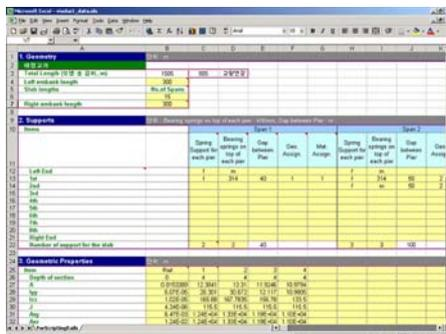
Spreadsheet data is used to generate model geometry automatically
