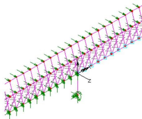
Exploded view of part of the LUSAS model showing embankment support and beginning of first span
